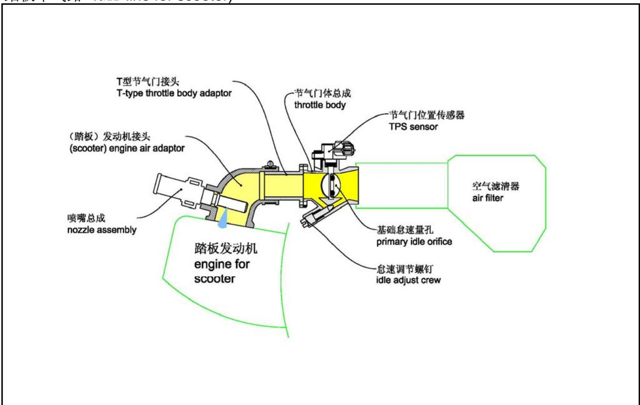
踏板车油路安装图 (illustration of fuel line installation for scooter)
